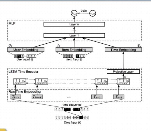
To capture the complex temporal dynamics, we utilize LSTM to encode the evolving interactions.
